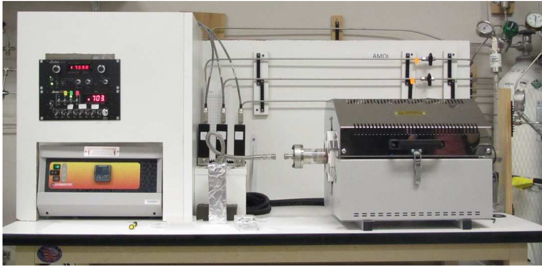
Figure 2.1 The home-build CVD graphene growth system
